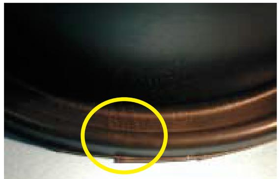
**Strike-through** is the amount of rubber that comes through the fabric to either fully or partially encapsulate the fabric during manufacturing.
